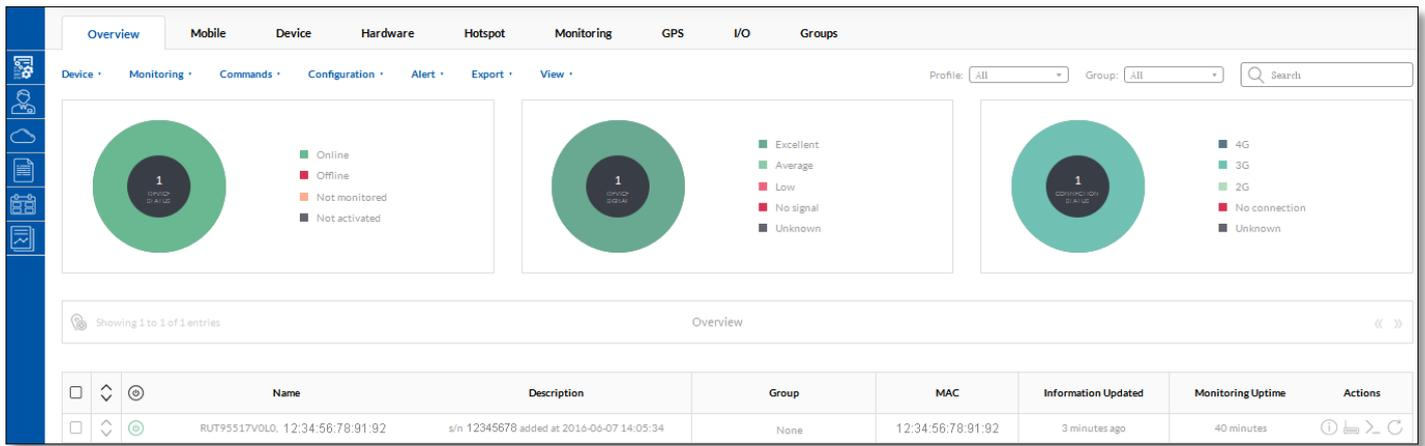
Via Overview -> Commands -> Access you can configure the attainment of the devices which are behind the router.
