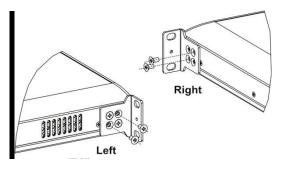
Figure 3-3 Securing Mounting Brackets
