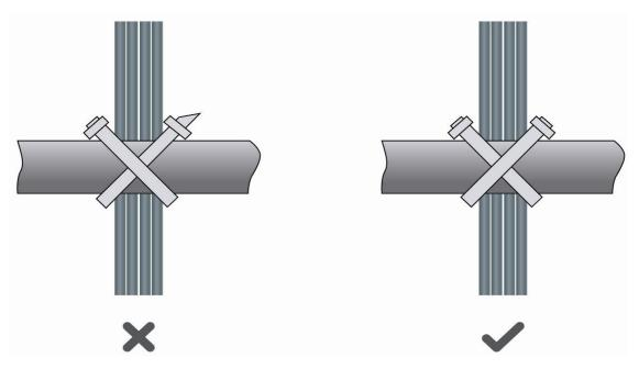
When cables need to be bent, please bundle them up but do not tie cable them where the cables will be bent, as shown in Figure D-3.
