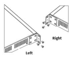
Step 4: As shown in Figure 3-4, horizontally mount the device to an appropriate position inside the rack and use M6 screws and cage nuts to secure the other end of the mounting brackets to square-hole posts of the rack.
