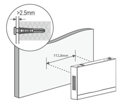
Figure 3-6 Mount the Switch on the Wall
