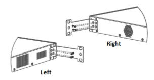
Figure 3-2 Securing Mounting Brackets
