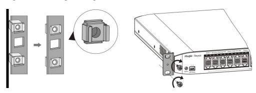
Figure 3-5 Securing Mounting Brackets
