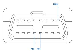
FMC800 OBDII socket pinout
