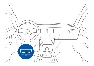
Most common OBDII connector locations.
