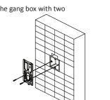
4 Align the device with the mounting plate, and secure the device on the mounting plate with 1 supplied screw (SC-KM3X6-T10-SUSS).
