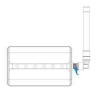
Note: Please do not let the front panel of products faces to walls if using embedded LoRa antennas.
