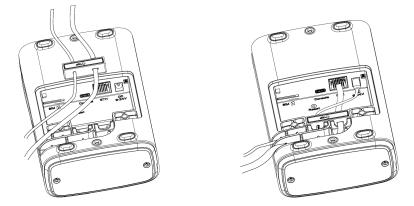
UG6x can also be powered by 802.3af standard PoE injector or other PoE devices. If both connected, DC power is preferred.
