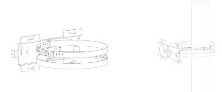
4. Screw the bracket fixing screws to the back panel of device, then hang the device to the mounting bracket on the pole.
