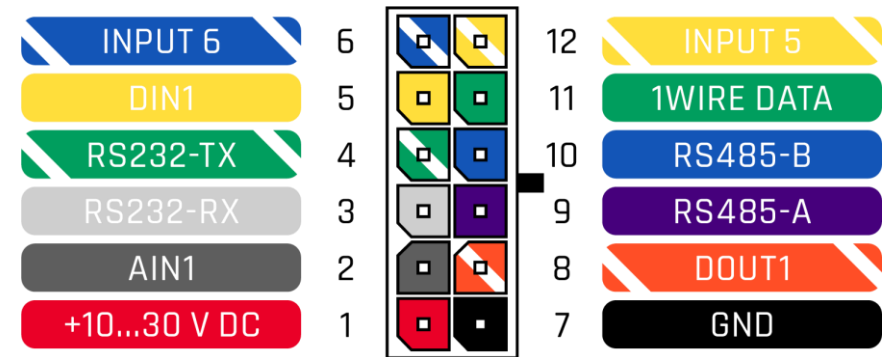
Figure 2 FMC125 2x6 socket pinout
