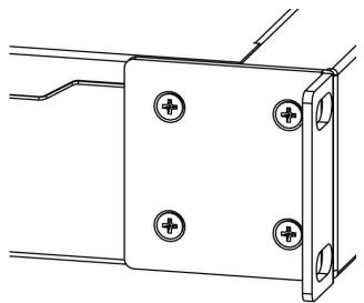
3. Tighten screws to secure it in place.
