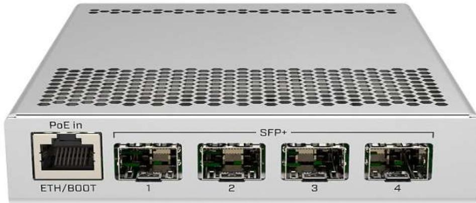
This device is a 10 Gigabit SFP+ switch, powered by RouterOS. It features two redundant DC inputs. The device has four SFP+ cages (modules are not included) for high-performance 10GbE connectivity (1.25 Gbit modules are also supported) and a 1GbE copper port for management. The device is ready to use as a switch.
